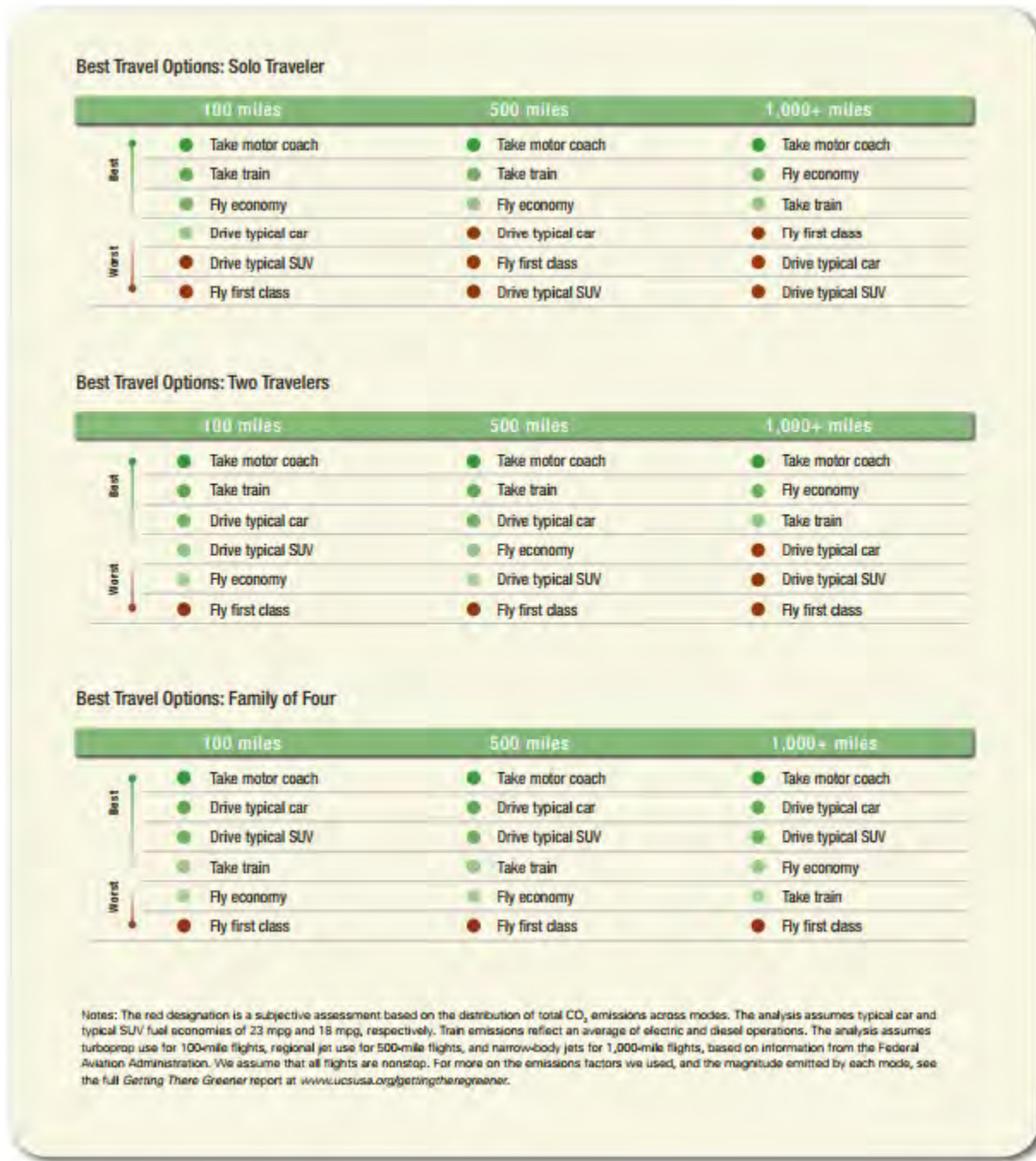
Figure 19-9: Relative Greenhouse Gas Emissions for Different Modes per Travel, by Group Size
